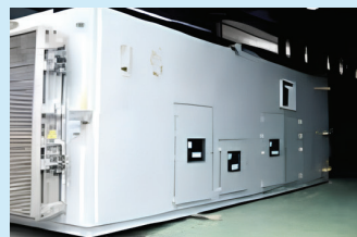
Generator set package for offshore platform
